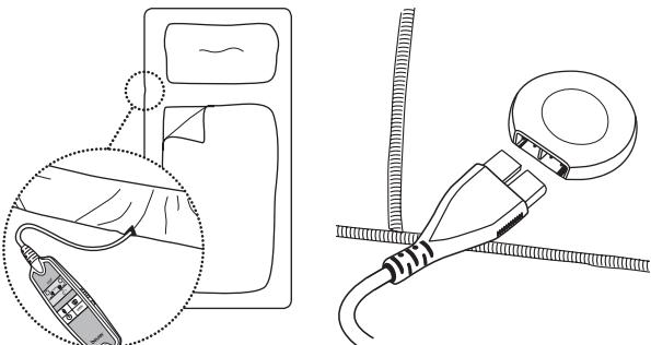
Then pull the side section over the sides of your mattress like a fitted sheet. The electric underblanket is designed to fit 90 x 200 cm as well as 100 x 200 cm mattresses. If the cable length is insufficient, you can order a longer power supply cord with the material number 108.424 from our specified Customer Service. Then fit your fitted sheet as usual with the electric underblanket positioned between your mattress and the fitted sheet.
